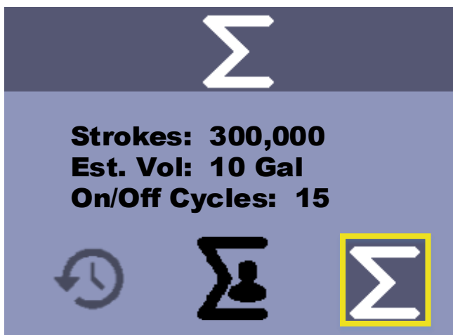
Figure 23: Pump Totalizer Screen
